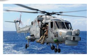
Helicopter: Agusta Westland Lenght: 15.16 m Height: 3.6 m Rotor diameter: 12,80 m Max take-off weight: 4,900 kg Speed : 324 km/h
