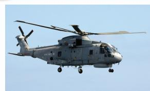
Helicopter: Agusta Westland Lenght: 22.81 m Height: 6.65 m Rotor Diameter: 18,6 m Max take-off weight: 14,600 kg **Speed :** 309 km/h or 150 kts Range: 1389 km
